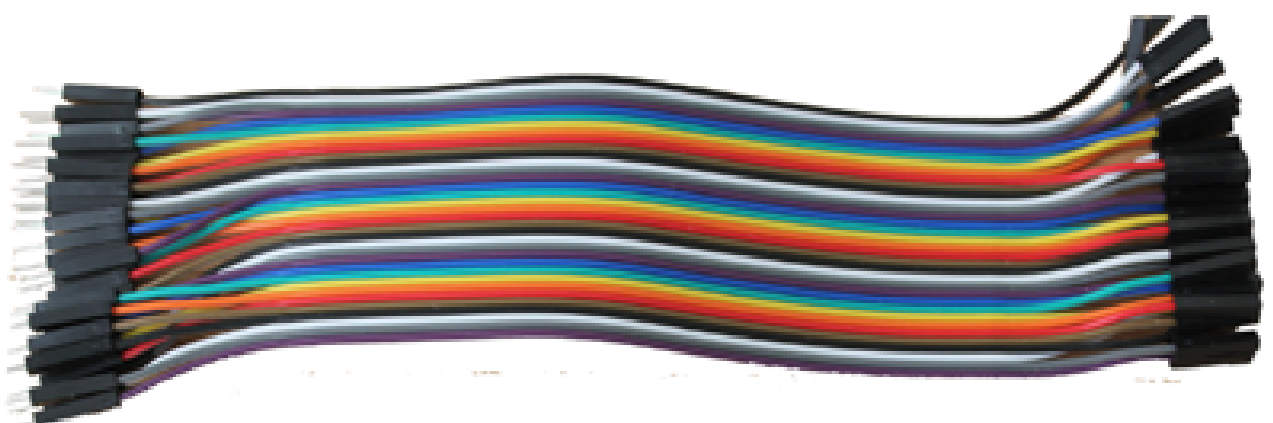
Jump Wires interconnect the components of a breadboard or other prototype
